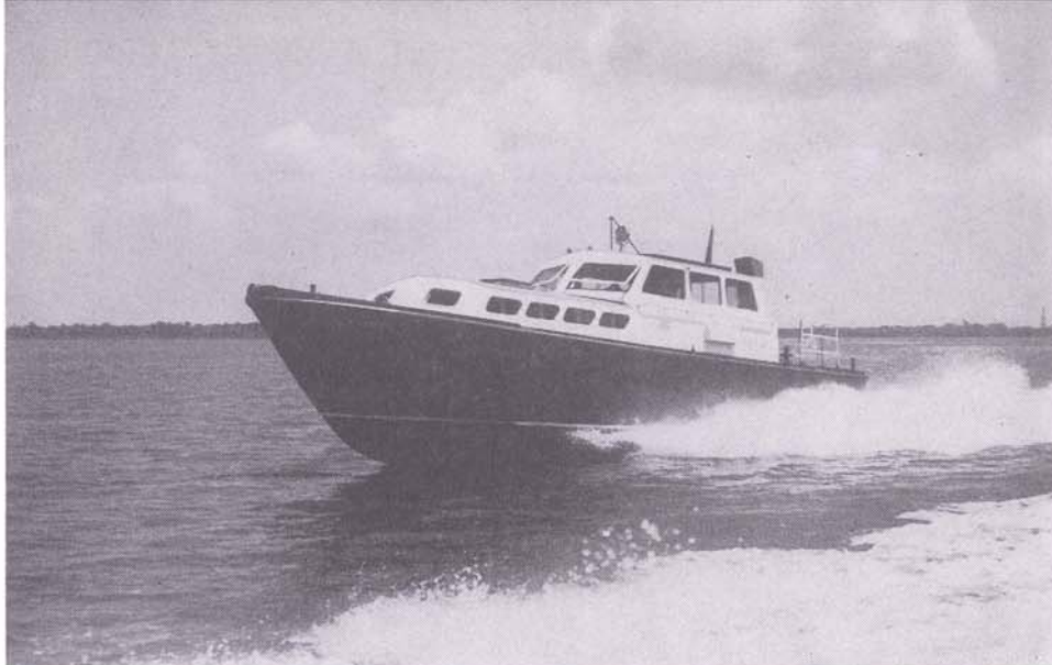
Typical of the crew boats which transport oil field workers to and from drilling sites in the tidelands is "Citation" above, photographed on a trial run on Lake Salvador in Jefferson Parish. She is an all-steel twin screw 48 footer powered by symmetrically matched turbo charged General Motors diesel engines. George Engine Company of Harvey, world's largest distributor of GM marine diesel engines, powered this speedcraft which has a top speed of almost 35 mph.
