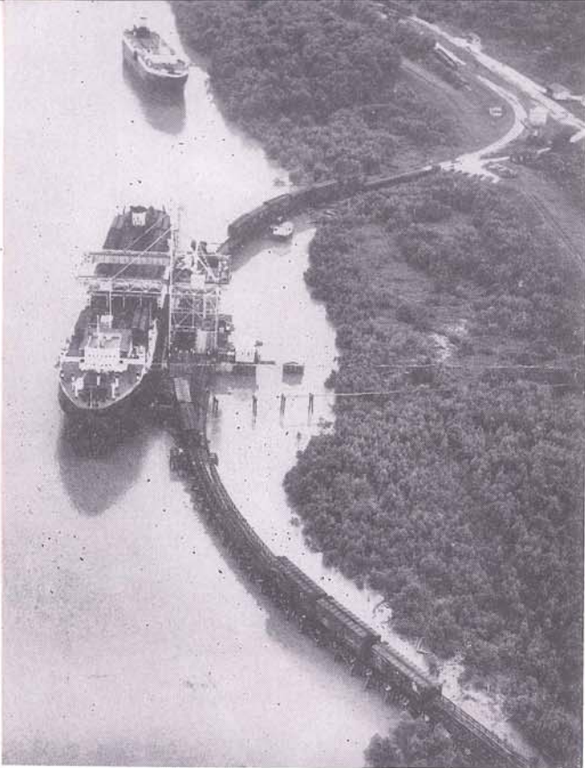
The always fascinating loading operation of the six Seatrain vessels that maintain weekly service between this dock at Belle Chasse in Plaquemines and the Port of New York. Each vessel will hold 100 fully loaded railway cars. The cars are lifted aboard on cradles by the 125 ton car lifting crane and lowered to any one of the four decks, each of which is four tracks wide. There is a total trackage of one mile on each vessel.
