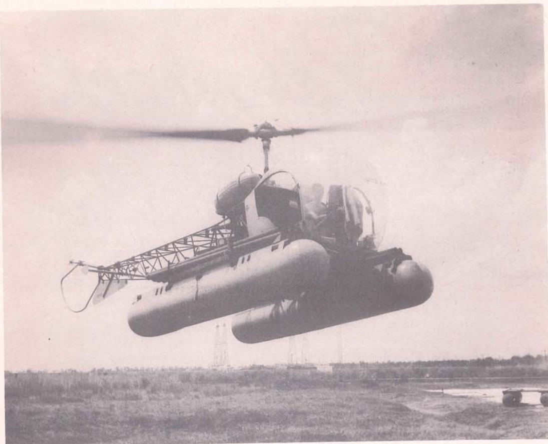
Pilot Frank Cady takes off with the greatest of ease, hangs poised while the Review photographer takes this picture, and then carries his load of pipe to location in a mere fraction of the time it would take a boat.
