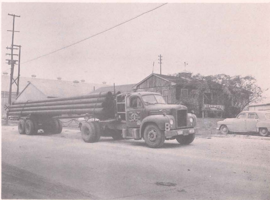
Trucking is another means of moving well casings from yard to location. Here is 17 tons . . . 20 joints of 10¾" surface casing going to Humble Oil & Refining Company's Paradis District in neighboring St. Charles Parish. Intracoastal Terminal, Inc. was in charge of the loading operation.
