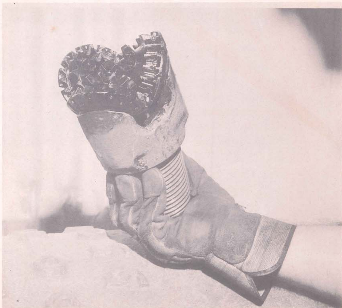
This is a drilling bit. As many as 12 different types may be used in drilling an oil or gas well. The bit is one of the more than fifteen thousand items carried in stock by Standard Supply and Hardware Company, Inc. on the east side of Harvel Canal.
