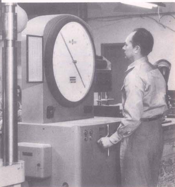
Modern precision machinery helps Palmer and Baker Engineers, Inc. lay the groundwork for planning the Jefferson Parish of tomorrow. Here a technician works at a machine testing the tensile strength of materials.
