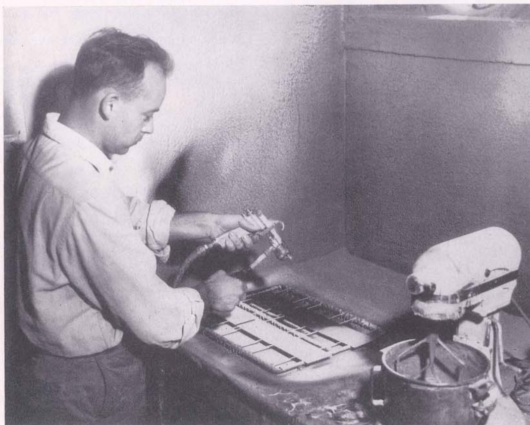
At Products Research Service, which manufactures marine finishes and industrial coatings and which is Plaquemines' newest industry, a chemist is shown test coating steel samples.
