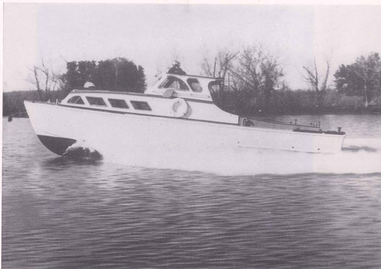
The first triple-screw high speed crew transport, designed by George Engine Company of Harvey for the inshore and offshore use of oil companies operating in Louisiana waters. The boat was completed, inspected and certified by the U. S. Coast Guard for 22 men in February of 1955. Reports from the field indicate complete satisfaction. The TRIPOD is 45 feet long with a cruising speed of 22 miles per hour and a top speed of 25.7 m.p.h.
