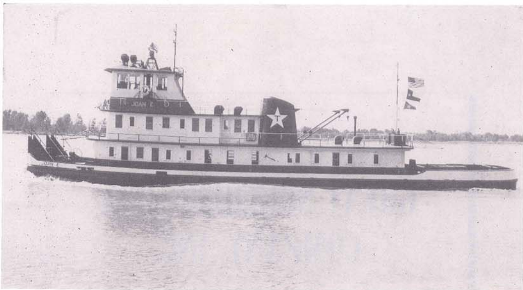
TWIN-SCREW towboat, "M/V Joan E", built by the Avondale Marine Ways for the Texas Towing Co., of Houston. Avondale has two yards, on river and on Harvey Canal, builds tuna clippers and other craft.
