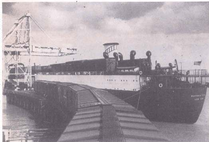
The five ships of the Seatrain line transport 100 loaded boxcars each, right to the dockside tracks in New York, Havana, Texas City, New Orleans.
