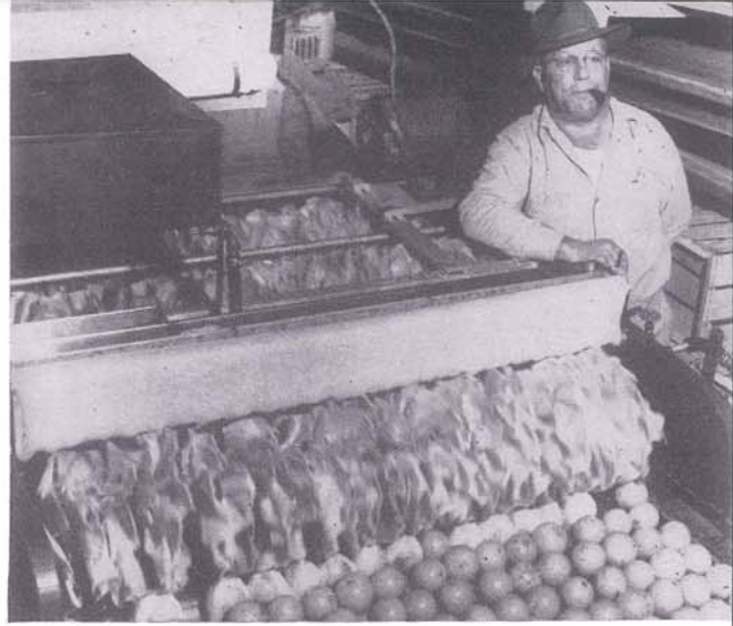
SLICK AND GLOSSY, delicious Louisiana oranges roll out of the waxing machine perfected by Anthony Commander, Jr., of Buras, who has worked also on other inventions beneficial to the orange industry.
