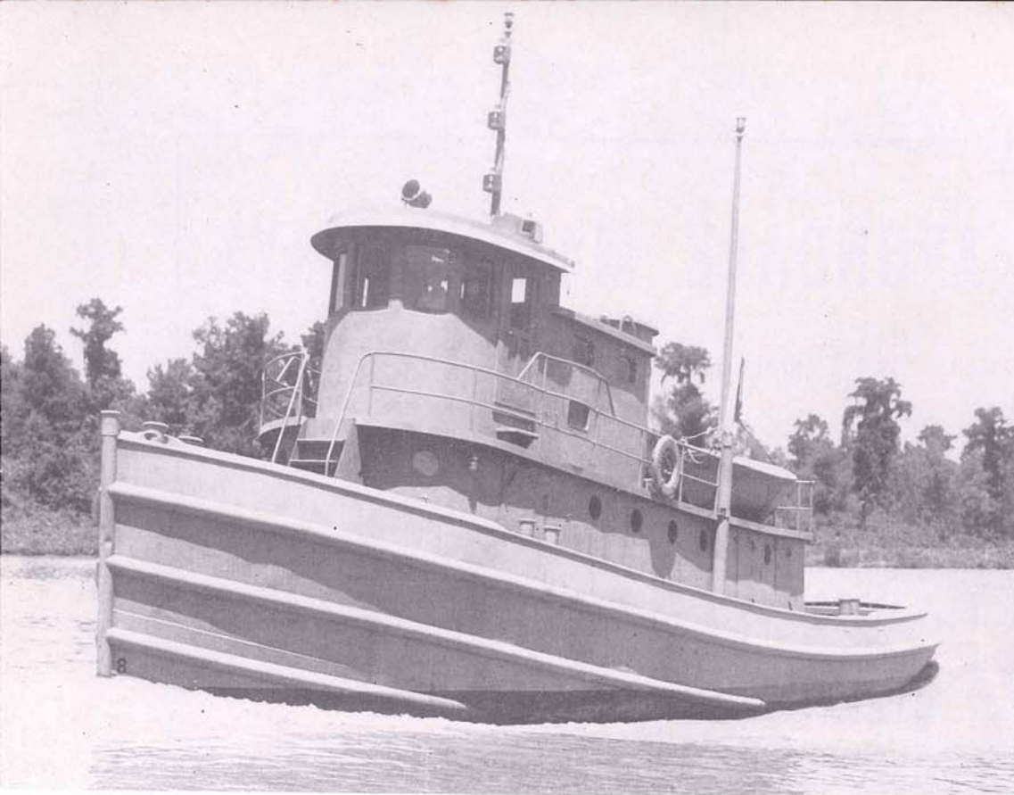
The Alboco, 76' all-welded steel tug built by Allen Boat Company, Inc., in May, 1942, for inland and coastwise service. Powered by a 320 horsepower Washington Diesel motor, she has an auxiliary Diesel generator, five pumps, electric refrigeration, steam heat, and crew's quarters for eight men.
